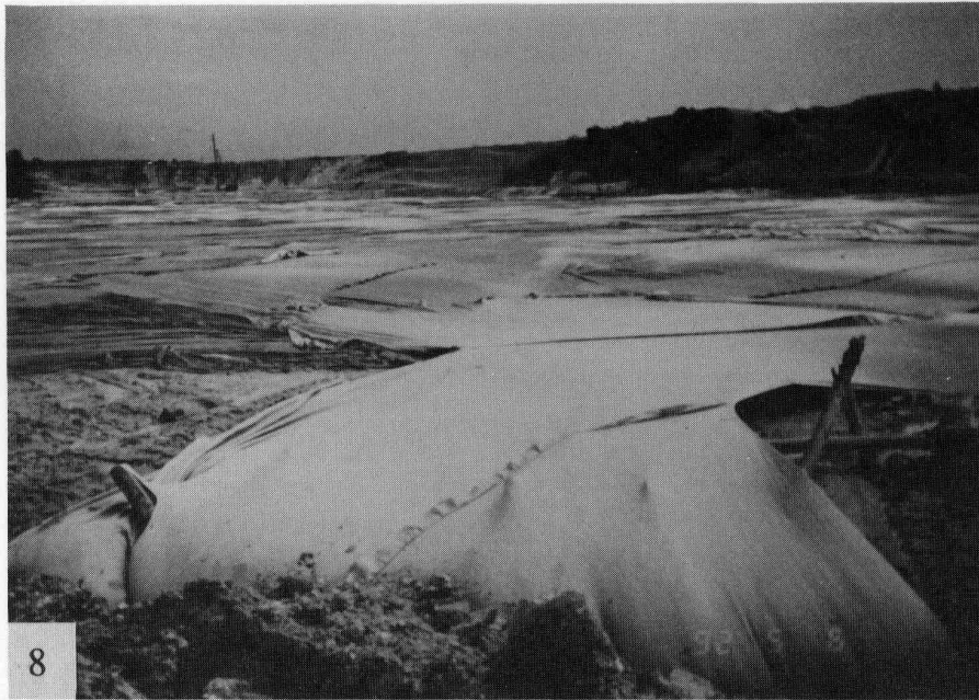
Fig. 8. Seam tearing and puncture of geotextile.
